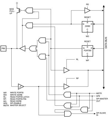
Figure 56. Port B Schematic Diagram (Pin PB6)
