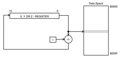
The X-, Y-, or the Z-register is incremented after the operation. Operand address is the content of the X-, Y-, or the Z-register prior to incrementing.
