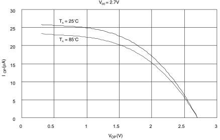
PULL-UP RESISTOR CURRENT vs. INPUT VOLTAGE  $V_{cc}$  = 2.7V
