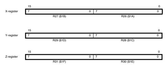
In the different addressing modes, these address registers have functions as fixed displacement, automatic increment and decrement (see the descriptions for the different instructions).
