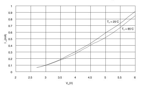
ANALOG COMPARATOR CURRENT vs. V<sub>cc</sub>
