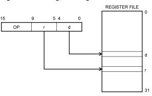
Operands are contained in register r (Rr) and d (Rd). The result is stored in register d (Rd).
