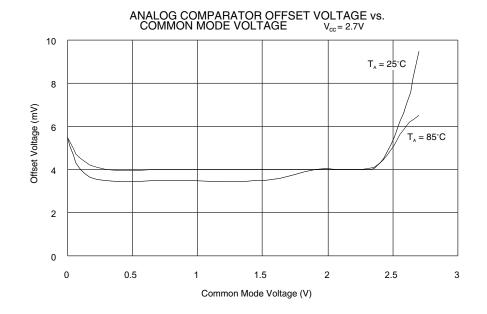
Figure 84. Analog Comparator Offset Voltage vs. Common Mode Voltage
