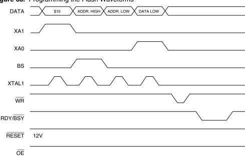
Figure 68. Programming the Flash Waveforms
