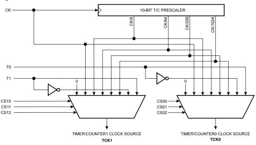
For Timer/Counters 0 and 1, the four different prescaled selections are: CK/8, CK/64, CK/256 and CK/1024, where CK is the oscillator clock. For the two Timer/Counters 0 and 1, CK, external source and stop can also be selected as clock sources.
