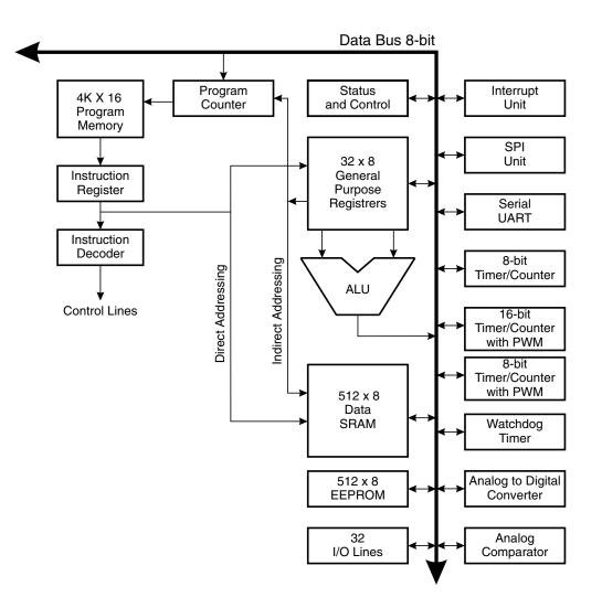
Figure 4. The AT90S8535 AVR RISC Architecture
