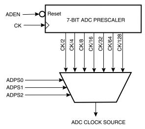
The successive approximation circuitry requires an input clock frequency between 50 kHz and 200 kHz to achieve maximum resolution. If a resolution of lower than 10 bits is required, the input clock frequency to the ADC can be higher than 200 kHz to achieve a
