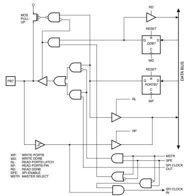
Figure 57. Port B Schematic Diagram (Pin PB7)
