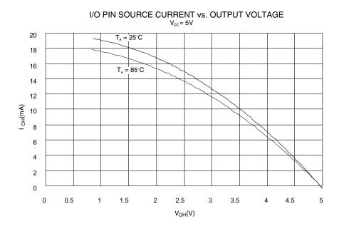
Figure 90. I/O Pin Source Current vs. Output Voltage
