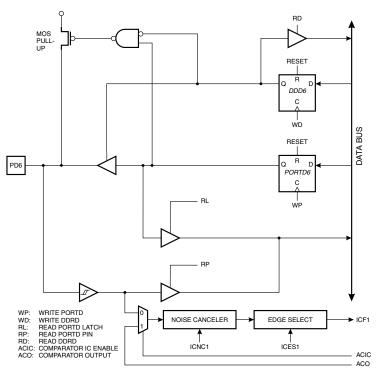
Figure 66. Port D Schematic Diagram (Pin PD7)
