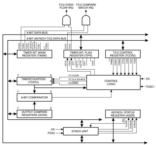
The 8-bit Timer/Counter2 can select clock source from PCK2 or prescaled PCK2. It can also be stopped as described in the specification for the Timer/Counter Control Register (TCCR2).
