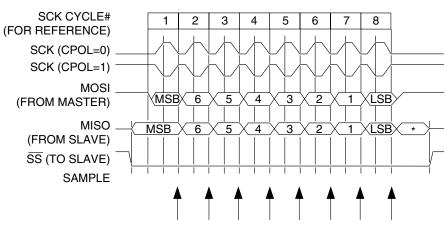
Figure 39. SPI Transfer Format with CPHA = 0 and DORD = 0
