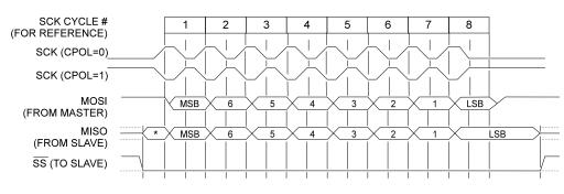
**Figure 40.** SPI Transfer Format with CPHA = 1 and DORD = 0
