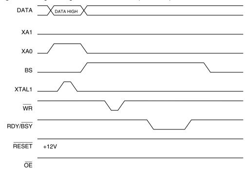
Figure 69. Programming the Flash Waveforms (Continued)
