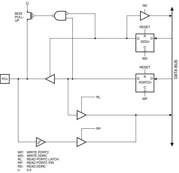
Figure 59. Port C Schematic Diagram (Pins PC6)
