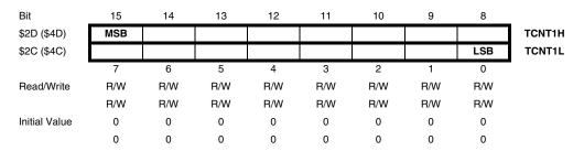
This 16-bit register contains the prescaled value of the 16-bit Timer/Counter1. To ensure that both the high and low bytes are read and written simultaneously when the CPU accesses these registers, the access is performed using an 8-bit temporary register (TEMP). This temporary register is also used when accessing OCR1A, OCR1B and ICR1. If the main program and also interrupt routines perform access to registers using
