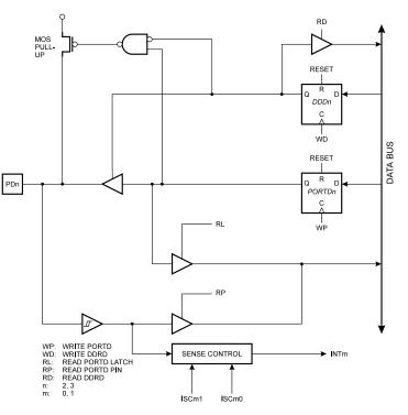
Figure 64. Port D Schematic Diagram (Pins PD4 and PD5)
